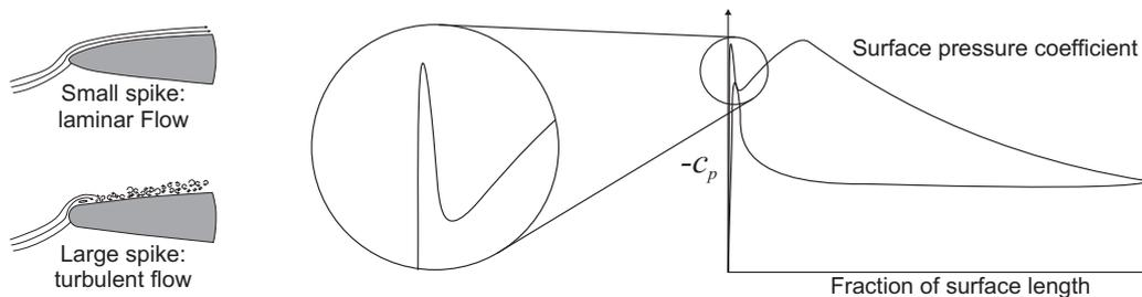
**Figure 2: Schematic of surface pressure distribution with enlargement of spike**
