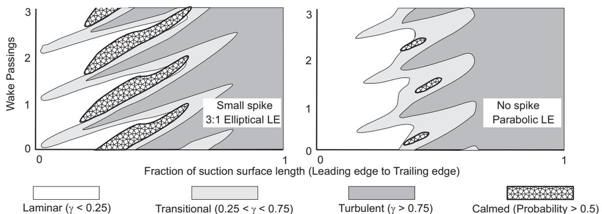
**Figure 3: The effect of small spikes on transition: Contours of time-resolved suction surface transition process at design incidence**
