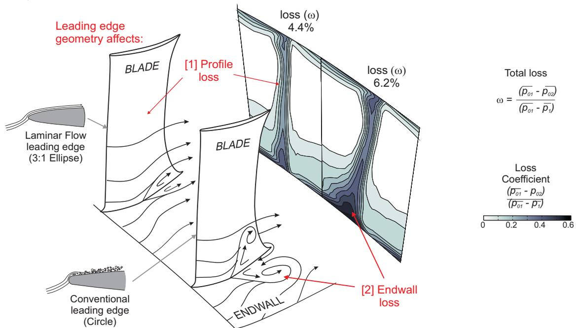
Figure 1 – The benefit of laminar flow leading edges: Schematic of surface limiting streamlines and plots of stagnation pressure deficit measured downstream.
